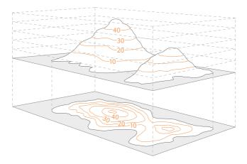
The picture shown illustrates how a landscape can be converted into contour lines on a map. An easy way to understand and visualise contour lines is to think of them as high tide lines that would be left by the sea. As the water level drops it would leave a line every 10 metres on the landscape. These marks would be contour lines.
