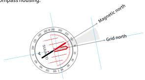
Compass readings are also affected by the presence of iron and steel objects, so be sure to look out for – and stay away from – pocket knives, belt buckles, mobiles and so forth when using your compass.
