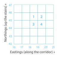
For example, the number 2 in the diagram is 19 across and 45 up and therefore the 4-figure grid reference is 1945. The numbered squares on the diagram would have the following 4-figure grid references:
