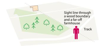
It's also possible to create transit lines using linear features such as walls, fences or straight streams, even if the features won't line up as they did above. By drawing lines on a map, extending the existing lines of linear features, you can create several transit lines that will help you pinpoint your location (as shown below).
