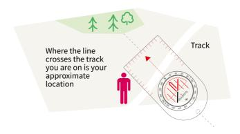
This bearing is a magnetic bearing rather than a grid bearing, which your map uses. You need to deduct magnetic variation from the compass reading to convert it. The magnetic variation is currently 0° to 5° throughout Great Britain (this amount changes annually, so check your OS map to work out the most current value).
